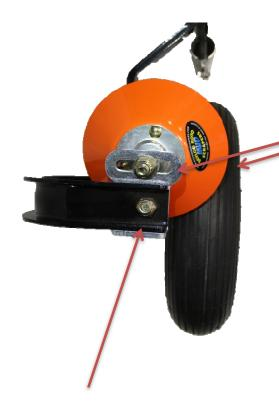
Adjust the scraper here to keep it 18 MM away form the edge of the tire.
