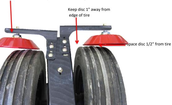
Due to the fact that Amity has their tires offset, we have extra holes and moon shaped slots to adjust the scrapers according to the angles of the tires
