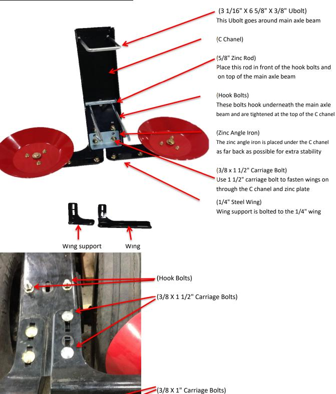
These are used to fasten the wing support to the wing
