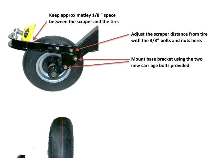
Slide the scraper in the slot so that it is offset minimum 3/4" from the edge of the tire on a 4" wide tire like this one.
