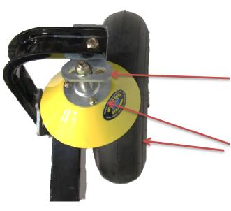
The zinc angle bracket with the slot is fastened to the "C" Channel with a 1" carriage bolt and nut.
