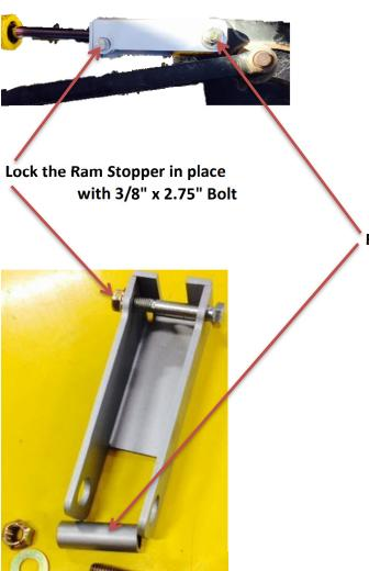
Replace pin with pipe bushing and 1/2 x 3" Bolt
