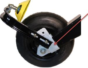
NOTE: There is two positions to mount the "C" chanels. The position leaning back is only used to avoid hitting the frame. The forward / higher positon is the preferred position.
