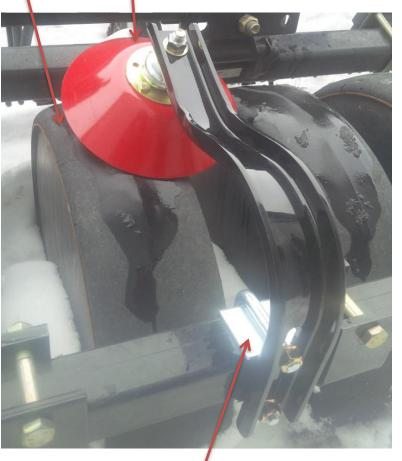
Put zinc channel over square tube and mount bracket on opposite side so that the tabs on channel fit into the slots on the bracket.
