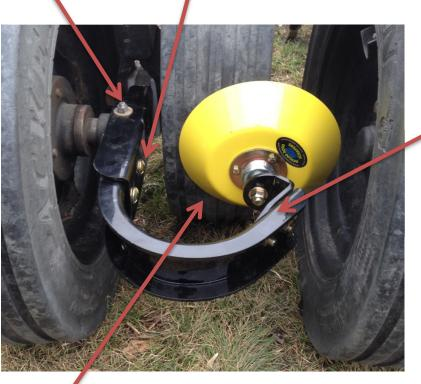
Angle bracket can be adjusted for front and back mounting
