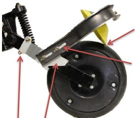
Adjust the scraper so that it has approximately 1/8" space between the tire.
