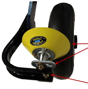
Slide the scraper in the slot so that it is offset minimum 3/4" from the edge of the tire on a 4" wide tire like this one.
