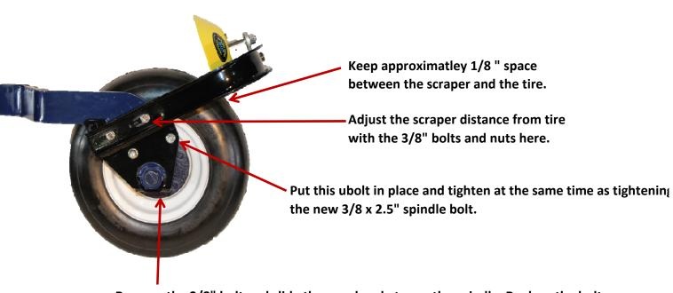
Remove the 3/8" bolt and slide the new bracket over the spindle. Replace the bolt with the longer  $3/8 \times 2.5$ " bolt provided. Make sure the ubolt is in place then tighten both to secure the base bracket.
