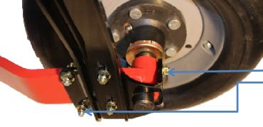
Remove the 3/8" bolt and slide the new bracket over the spindle. Replace the bolt with the longer 3/8" bolt provided.
