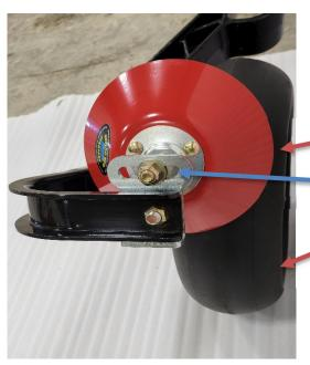
4. Make sure to place the scraper 3/4 inch from the edge of the tire to increase performance.
