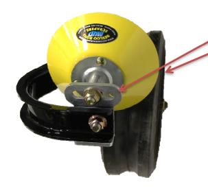
Use a straight edge (Carpenters Square) and adjust the scraper in the slot so that the scraper is at 3/4" from the side of the tire.
