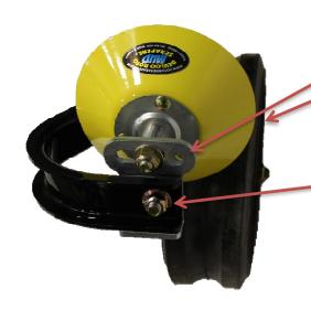
Use a straight edge (Carpenters Square) and adjust the scraper in the slot so that the scraper is at 1/2" minimum from the side of the tire.
