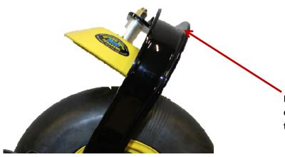
Mount the upper bracket with the two 3/8 carriage bolts loosely before mounting the lower bracket on the seeder.
