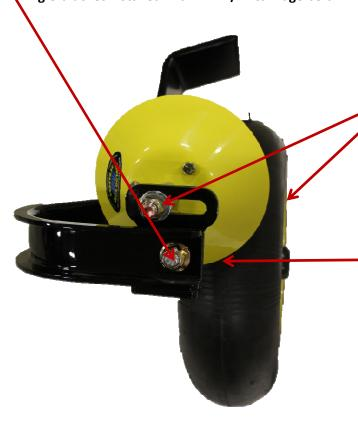
Use a straight edge (Carpenters Square) and adjust the bolt so the scraper is 3/4" minimum from the side of tire.
