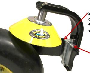
Slide the zinc plate tight in the corner of the Seed Hawk opener arm bend using the 7/16 ubolt and nuts to fasten it in place so that there is approximately 1/8" space between the tire and the scraper.
