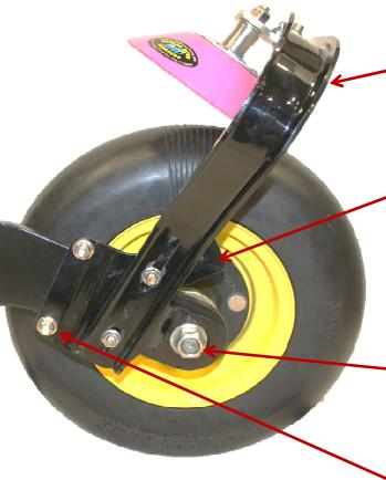
Mount the upper bracket with the two 3/8" carriage bolts loosely before mounting the lower bracket on the seeder.
