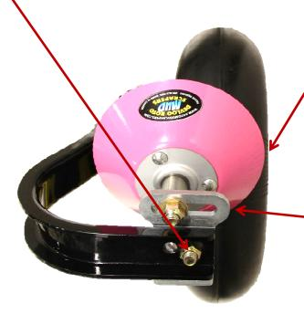
Use a straight edge (Carpenters Square) and adjust the scraper in the slot so that the scraper is at 3/4" minimum from the side of the tire.
