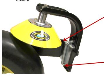
Slide the zinc plate tight in the corner of the Seed Hawk opener arm bend using the 7/16 ubolt and nuts to fasten it in place so that there is approximately 1/8" space between the tire and the scraper.
