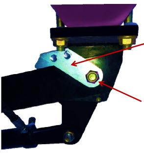
If there are spots on the seeder that the scraper will still hit the frame or hoses, we use this zinc stopper to stop the opener from coming all the way up.
