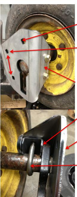
There are two positions to mount the upper bracket to the base bracket. This is determined by the angle you need in order to have the scraper miss the frame
